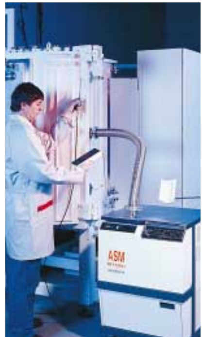
Leak testing of a 1000 liters chamber on a sputtering system with ASM 181 T2D+
